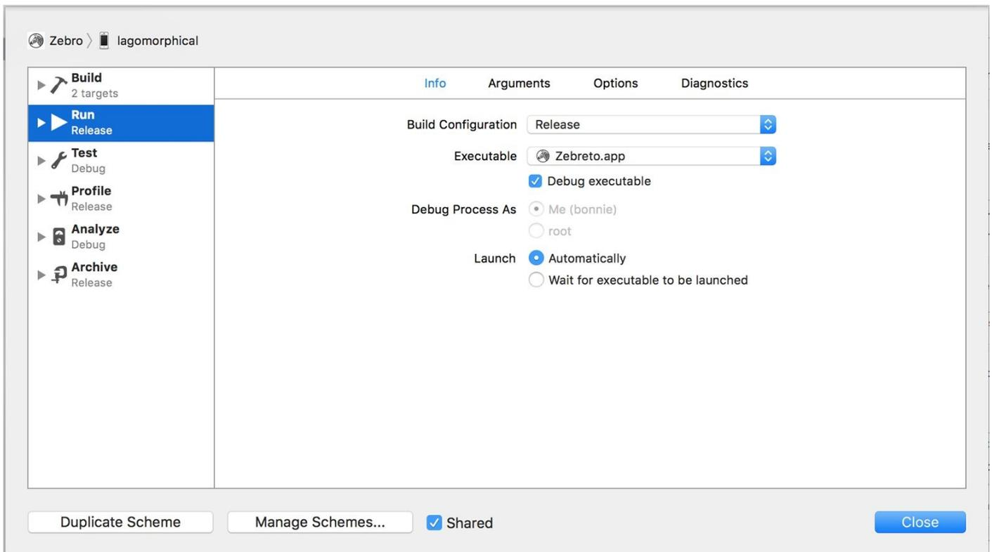
Figure 10-12. Set the Build Configuration to Release and uncheck “Debug executable”
