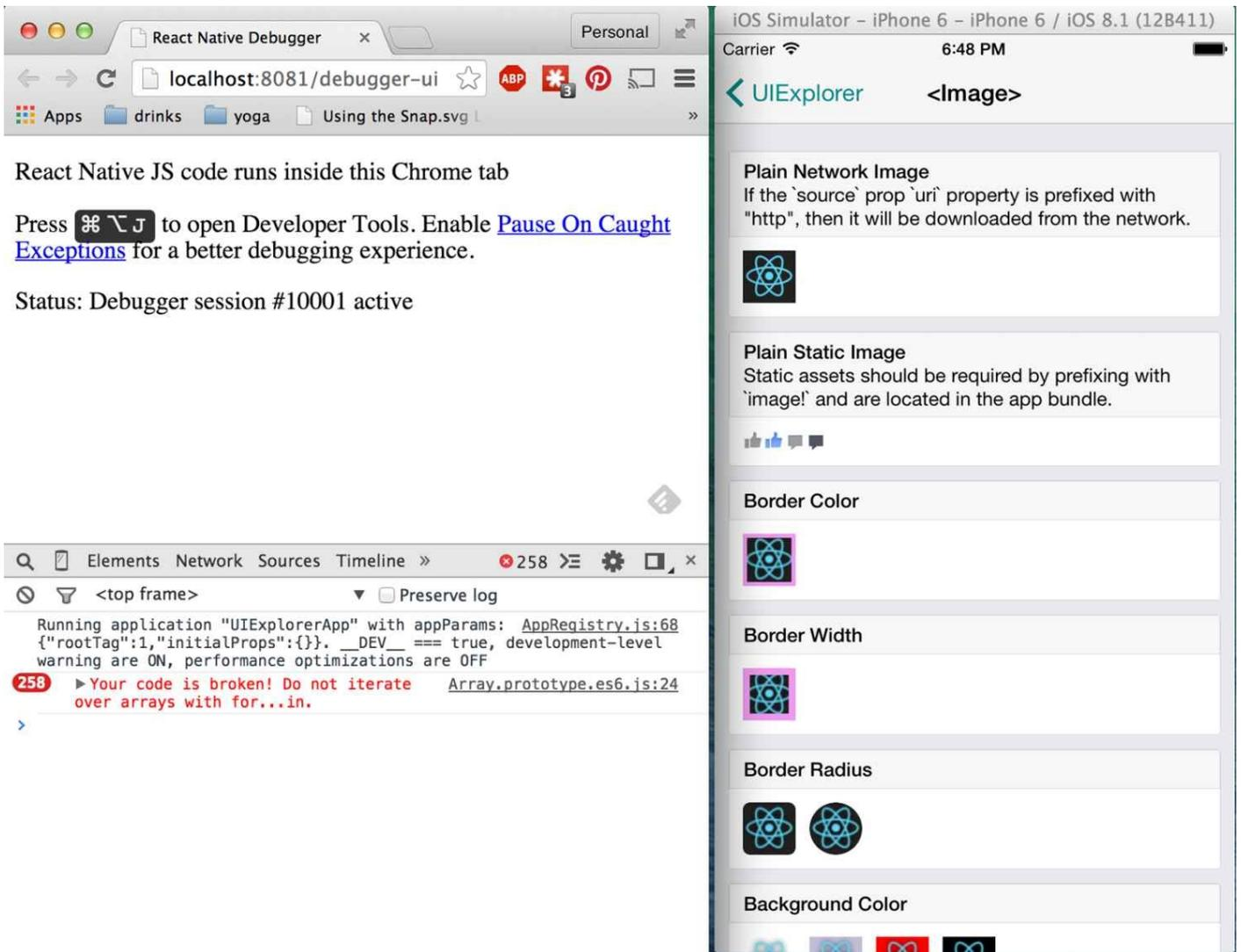
Figure 1-1. Using the Chrome Debugger
