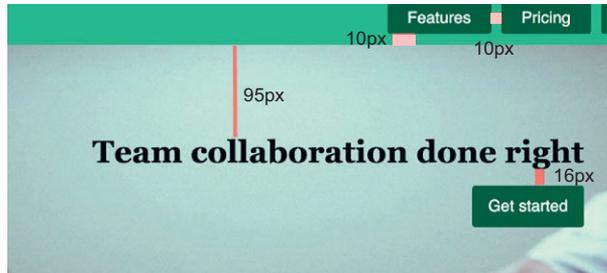
**Figure 12.19** The design calls for 95 px above the slogan and 16 px beneath it (between it and the button).
